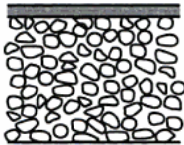
Figure 3: The cross section of a thin film composite anisotropic membrane (Baker, 2004).
