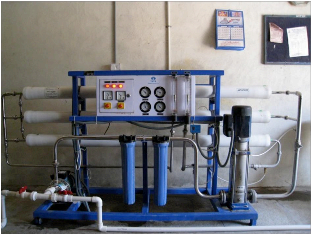
Picture 2: Shows a TATA plant with capacity of 1m 3 /h (Havig and Holstad, 2010).
