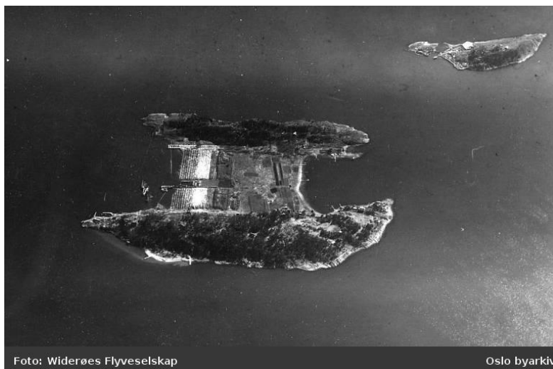
Picture 1: Langøyene ca 1937 seen from air. We see how the two islands are connected with the landfill. Oslo Municipality sank old ships to dam the waste. Source: (Widerøes 1937)
