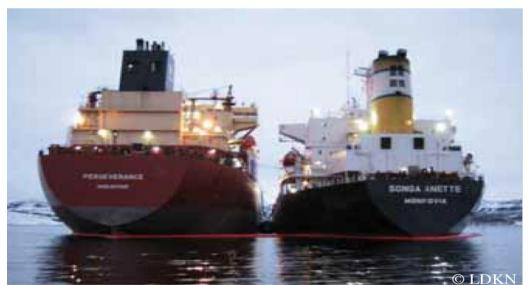
Figure 52: Ship-to-Ship transfer operations of fuel, oil cargo. Source: (Bambulayk 2009, 62)
