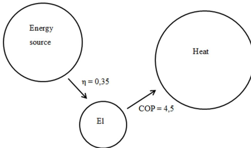
**Figure 5.1 Lost and gained useful energy when converting fossil fuel to heat via electricity and heat pump.**
