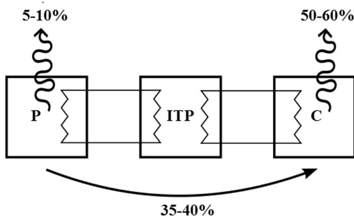
**Figure E-1 District heating system with heat producer (P), individual heat station (ITP) and consumer (C). In Ukraine heat is transferred directly from producer to consumer. Estimated losses are illustrated at each point**
