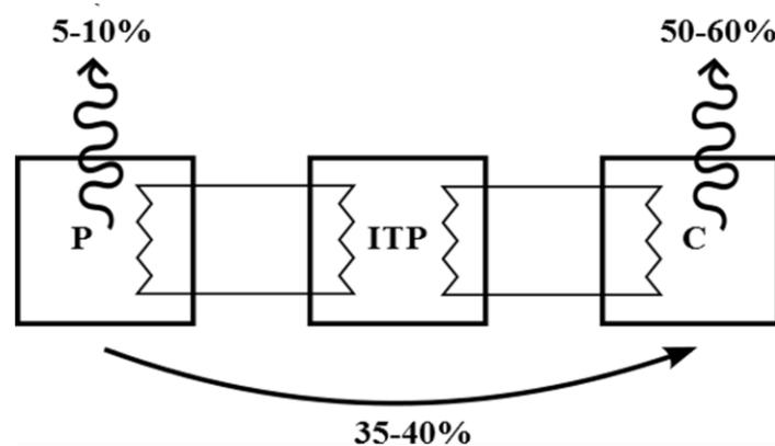
**Figure 2.2 District heating system with heat producer (P), individual heat station (ITP) and consumer (C). In Ukraine heat is transferred directly from producer to consumer. Estimated losses are illustrated at each point (Ivanenko & Petryna 2012)**
