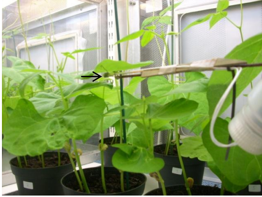
Picture 2. The sensors of the Modular Signal Recorder were located underneath the leaf. Photo: Ronny Berdinesen.
