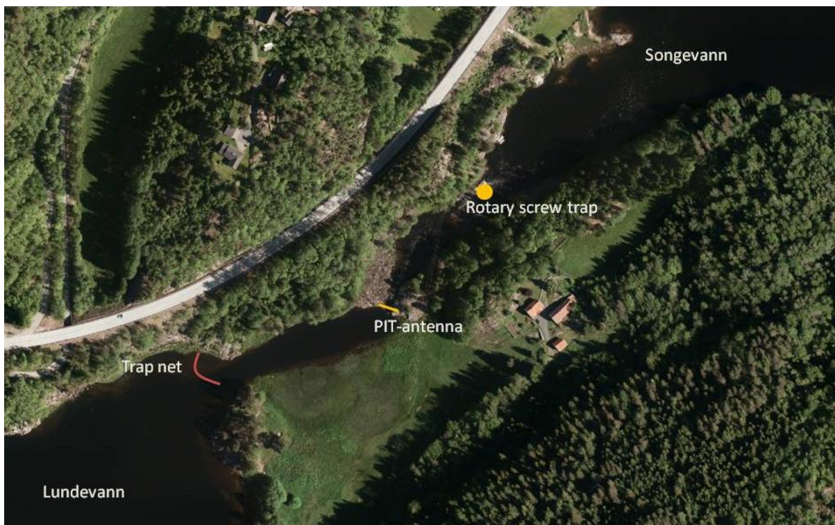
Figure 3: Position of the trap net in Lundevann with entrance facing towards the exit of the lake. The PIT-antenna was placed at the entrance of Strømmen and the rotary screw trap at the exit.
