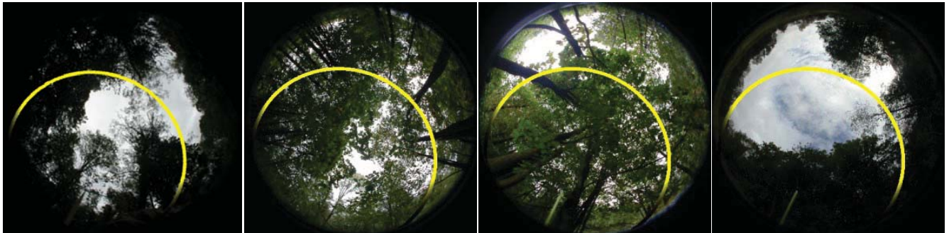
Figure 4. Wholesky pictures from a riparian strip in Lier including plotted sunpaths for the period of the field experiment. Left to right: 1-4.
