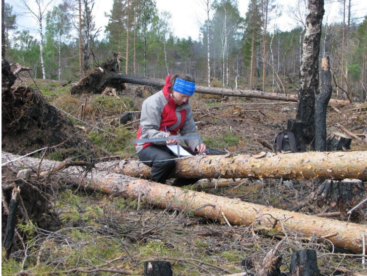
Figure 18. Recording diameter using a calliper (Photo: Per Holm Nygaard).
