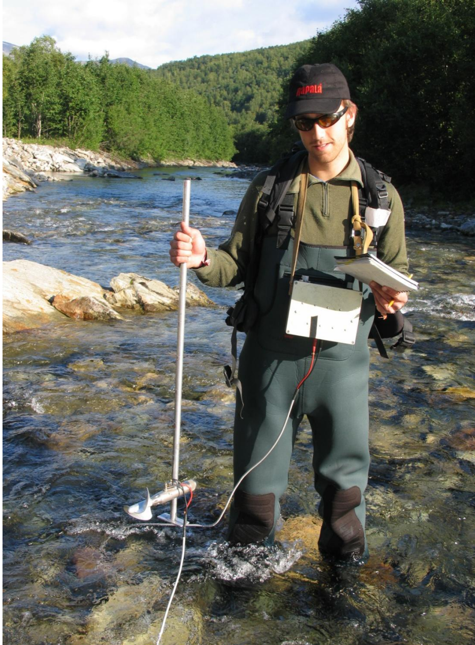
Figure 6. Author holding the C31 Universal Current Meter and a CMC-200 counter in the Bognelva river. Photo: Jonathan E Colman 2008.
