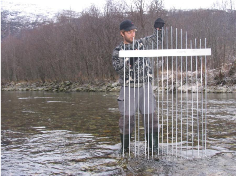
Figure 5. The contour/profile measurement device in use in the Bognelva river. Photo: Jonathan E Colman 2008.
