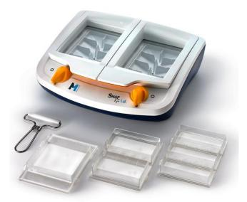
**Figure 3.5: The SNAP i.d. Protein Detection System**. The system is based on a vacuum-driven technology and a built-in flow distributor that actively drives reagents through the membrane. SNAP i.d. single well blot holder was used, but it exist three different sizes of blot holders. Two blot holders can be run in parallel in the system. The figure is taken from SNAP i.d. Protein Detection System protocol by Millipore
