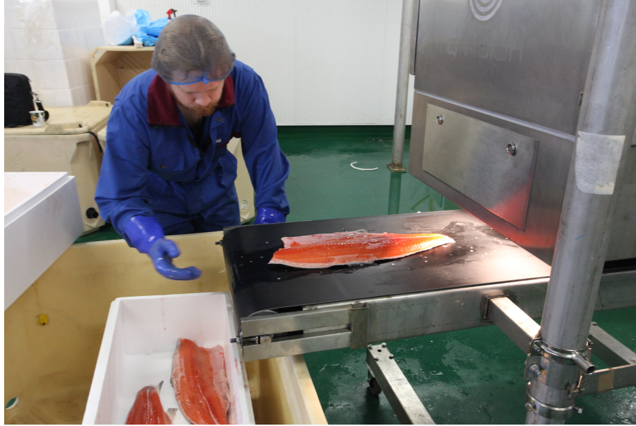
FIGURE 4.15: Measuring the fat using QMonitor in Stofnfiskur, Iceland
