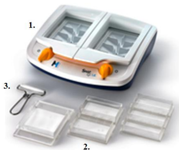
Figure 3. 4: The SNAP i.d. Protein Detection System. The SNAP i.d. system (1) consists of two independent blot holder stations. The system allows for blotting of up to six individual blots, using the different blot holders (2). Separately controlled blotting is possible by adjusting the vacuum of each station. The blot roller (3) is used for removal of air bubbles when placing the membrane in the blot holder. The illustrative figure is taken from the SNAP i.d Protein Detection System- protocol (Millipore)
