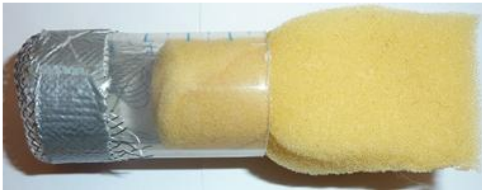
Figure 2: Arm cage. The wire mesh end was inserted into the T-maze to allow communication.
