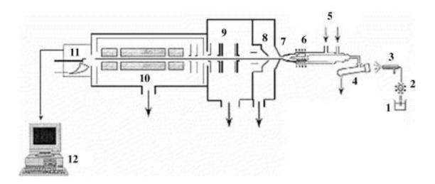
**Fig. 4.** Schematic diagram of inductively coupled plasma-mass spectrometer: (1) liquid sample, (2) pump, (3) nebulizer, (4) spray chamber, (5) argon gas torch inlets, (6) torch, (7) sampler cone, (8) skimmer cone, (9) ion lenses, (10) quadrupole mass analyzer, (11) electron multiplier detector, and (12) data collection (Nageswara Rao & Kumar Talluri 2007).
