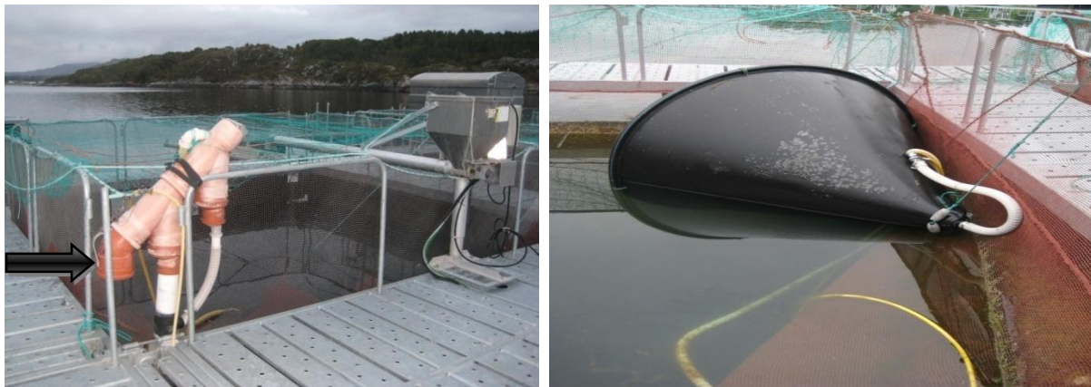
Figure 8 - Collector system of uneaten feed pellets at Nofima research station, Averoy, Norway (Photo: B.Rahnama)
