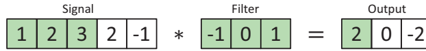
Figure 2.8: Illustration of the cross-correlation (flipped convolution) between a signal and a filter.
