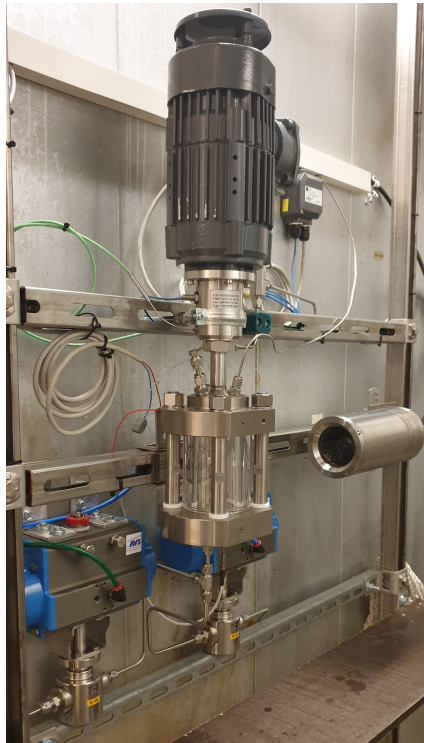
Figure 3.1: Wetting Index cell used for hydrate formation experiments with stirrer, temperature regulation, pump and camera. Picture by Martin Fossen.
