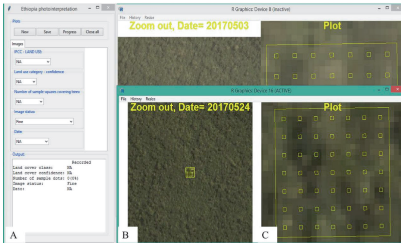
Figure 2. The graphical user interface used for visual image interpretation. (A) A window for opening new image and recording the interpreted data; (B) 1 \text{ km} \times 1 \text{ km} image with a point at the center; (C) a zoomed into 0.5-ha cell with the 49 points ( 2 \text{ m} \times 2 \text{ m} squares).
