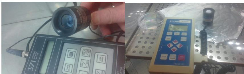
Figure 8. Picture to the left: Red light Detector-model 247, serial number 77079, with the instrument 371 Optical Power Meter, United Detector Technology. Picture to the right showing the blue light instrument and detector: Solar Light Co, PMA2100, Detector; Blue Light Safety, Solar Light Co, Philadelphia, Pennsylvania, Serial number; 2894. Photo: K.S. Pettersen, 2016.
