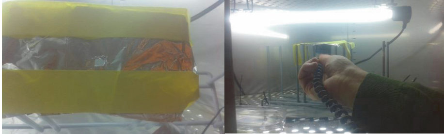
Figure 9. The picture to the left shows the 5×5 mm hole made for excluding all radiation coming from the sides when placing the detector just below the hole (picture to the right). Photo: K.S. Pettersen, 2016.
