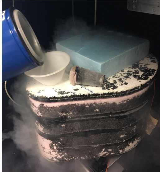
Figure 4.8: Filling the cryogenic cooler with liquid nitrogen.
