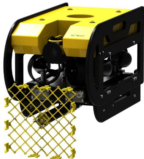
Figure 9 ROVeee with plastic mesh mounted in front.
