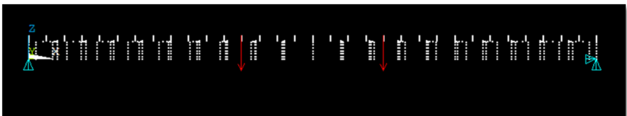
Figure 29 shows the applied loads as forces on nodes in the negative z-direction. The red arrows illustrate the forces.
