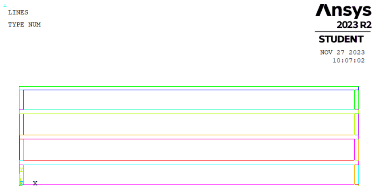
Figure 22 The plotted lines of the geometry for the beam-frame and the OSB, where they illustrate that the volumes are glued together.
