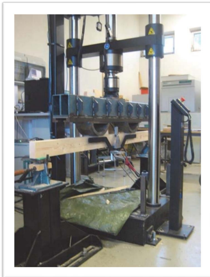
Figure 8 Machine from Instron 5800 applying four-points bending tests for the identifications of MOE and MOR. (Fischer, 2016).
