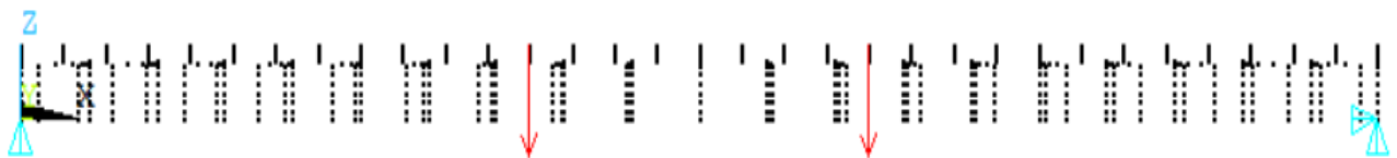
Figure 24 The constraints in the lower edges of the TCC floor system inside the ANSYS model. Nodes in the left edge restrained in Z-direction while in the right edge in both Z and X.
