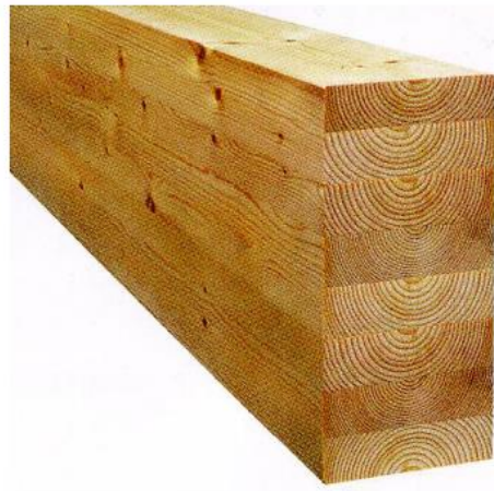
Figure 5 Glued laminated timber (Glulam) (Balb & Sandhaas, 2017)
