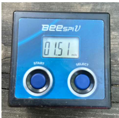
Fig. 2: The figure shows the speed gate reading screen. One can directly read the speed in meters per second for the outgoing ball in the Newton's cradle. In this particular reading, the speed of the outgoing ball was 1.51 meters per second.
