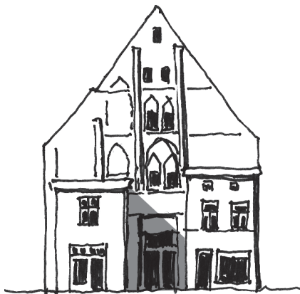
Mönchstrasse 38, schematic facade showing the ground floor store-extension increasing the sales-area. Sketch: Martin Ebert
