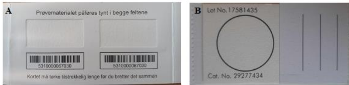
Figure 4 - BSC (A) with square sample fields and FTA-cards (B) with round sample field, used as a transport media for rabies spiked samples.
