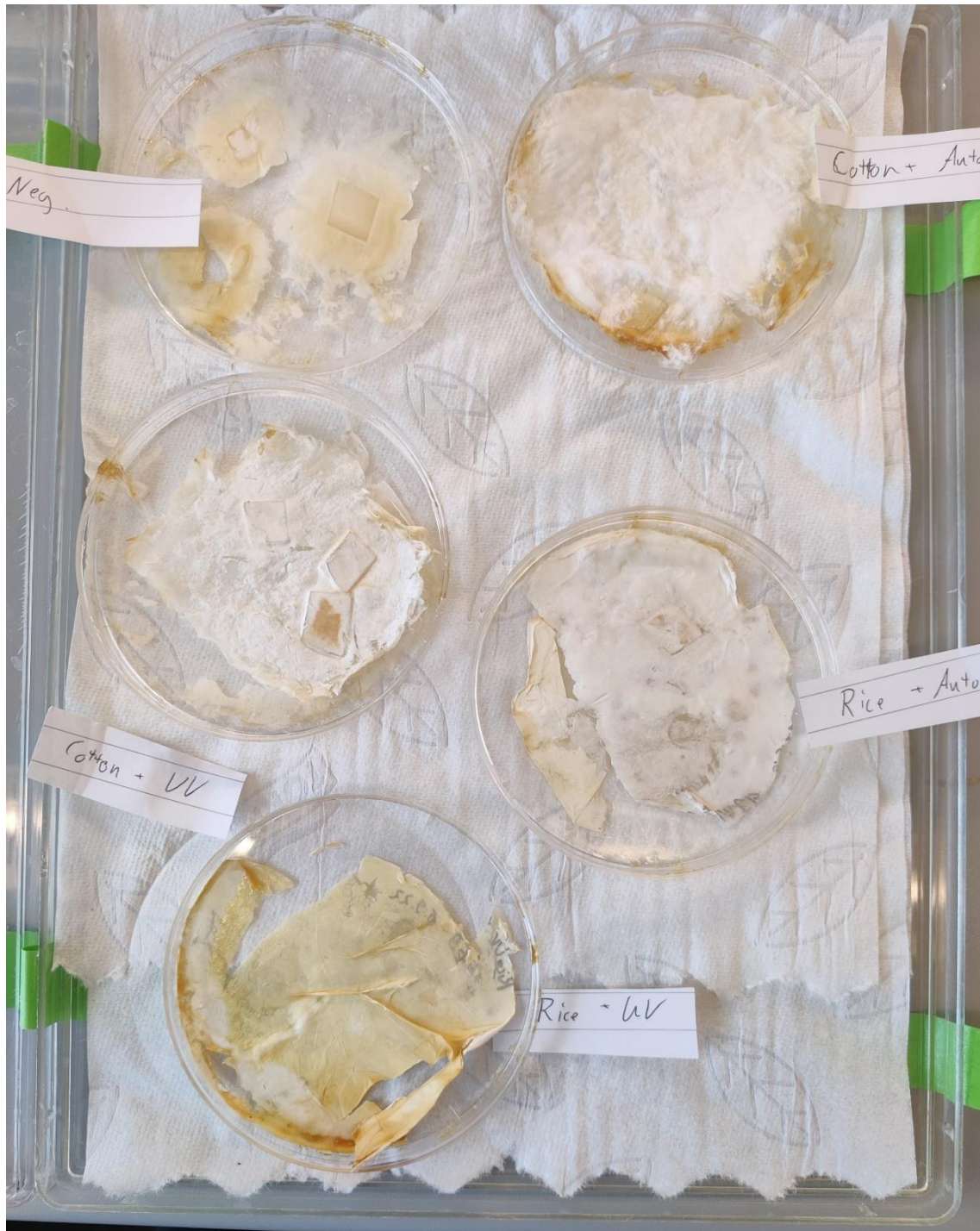
Figure 26 Pictures of dried and pressed Ganoderma lucidum mycelium. Neg indicates that the mycelium was grown in only MEB. Cotton indicates mycelium grown in cotton wool and rice indicates mycelium grown on rice paper. Auto indicates that the substrate, being cotton or rice paper, was treated by autoclave, or by UV exposure in the case of UV.
