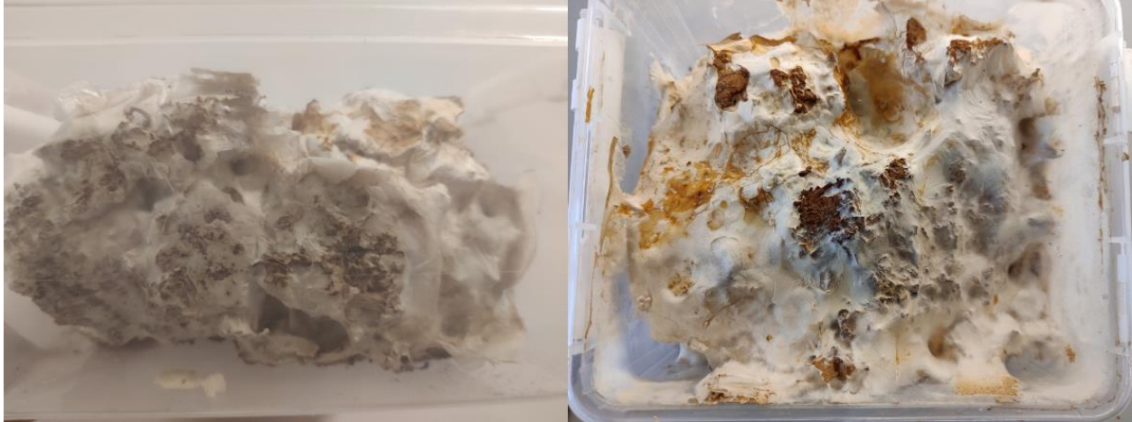
Figure 44 Picture of box containing spruce sawdust inoculated with F.p.-5 mycelium covered rye. The left picture is taken from the side, while the right is taken from the top.
