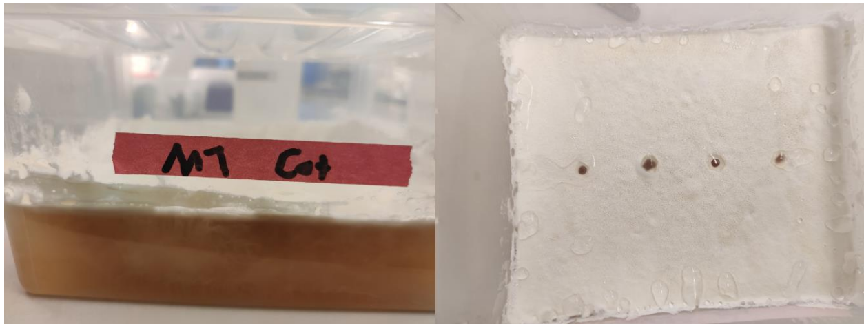
Figure 30 Picture of G.l.-1 grown in MEB on nylon tulle seen from the side (left) and seen from the top (right)
