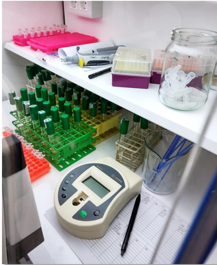
Figure 2.5. Illustration of physical conditions of anaerobic growth trials. All necessary equipment and growth media are brought inside the cabinet and removed of oxygen before inoculation with bacteria. The environment is kept constant anaerobic at 37 °C. Growth is measured with a portable spectrophotometer. Photo: Veronica Mehammer.
