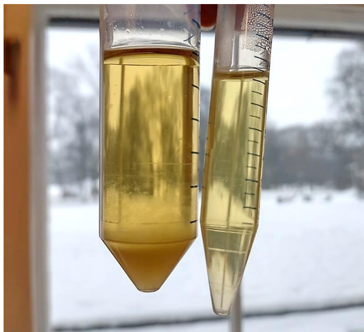
Figure 2.7. The visual solubility of deacetylated mannan versus native mannan. NaOH-treated spruce mannan to the left (10 mg/mL) and native spruce mannan to the right (50 mg/mL) in MQ water at 4 °C. Photo: Veronica Mehammer.
