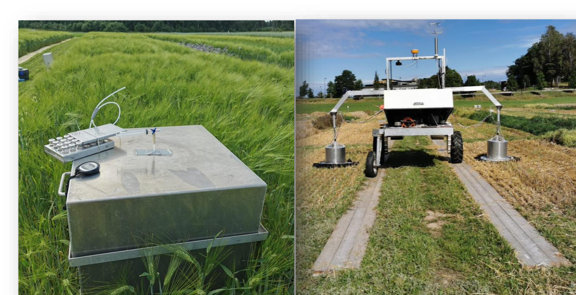
Fig.4 N 2 O measurements with manual chambers (left) or robot (right)
