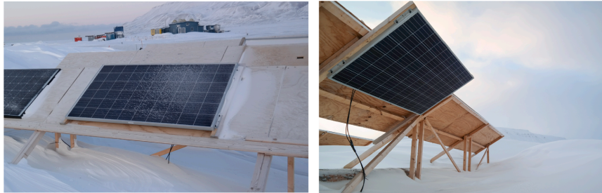
Fig. 2. Module installation with a sky-facing module (left) and a ground-facing module (right). The modules are lifted 2 cm from the wooden surface to allow for ventilation on the backside.
