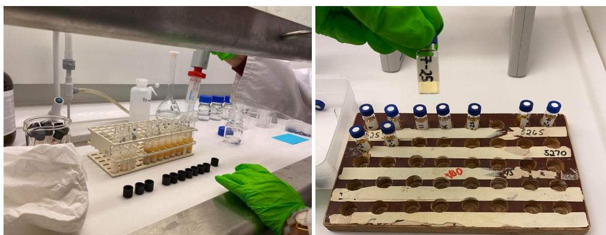
Figure 3.8. Addition of H_2SO_4 after cooling in cold water bath (left) and hexane layer siphoned into labelled GC vials for gas chromatography (right).
