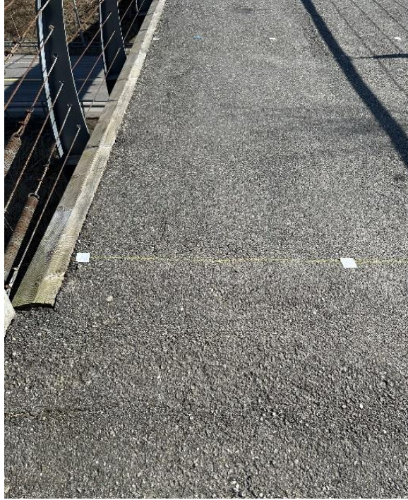
Figure 3.4: illustration of placement of the double-sided tape for securing the sensors.
