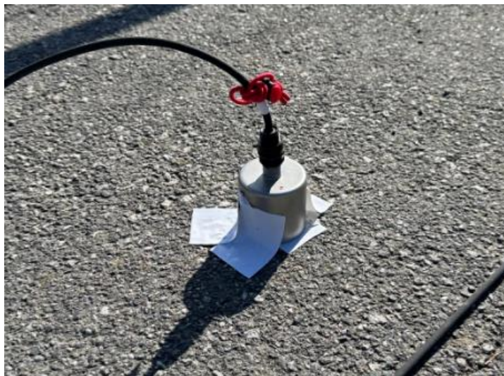
Figure 3.6: Reference sensor marked with a red ribbon.
