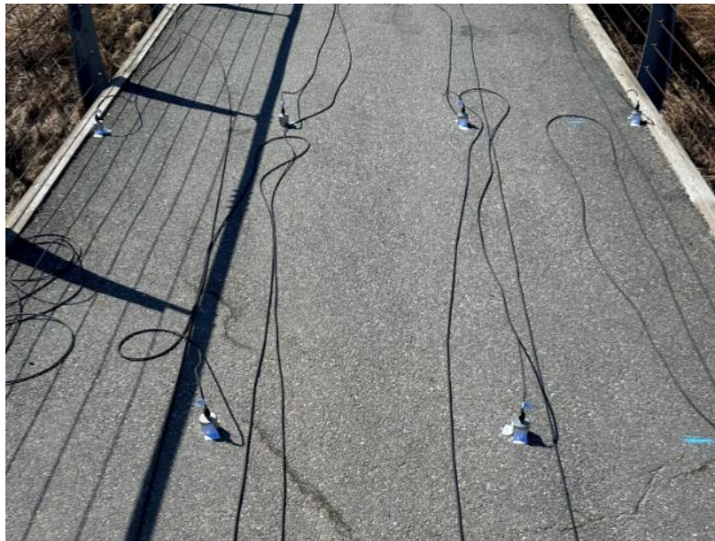
Figure 3.5: Distribution of the sensors on the timber bridge with the same spacing and distances.
