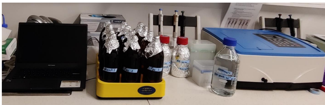
Figure 5. Experimental set-up for the measurement of PAA in water samples using a Spectrophotometer.
