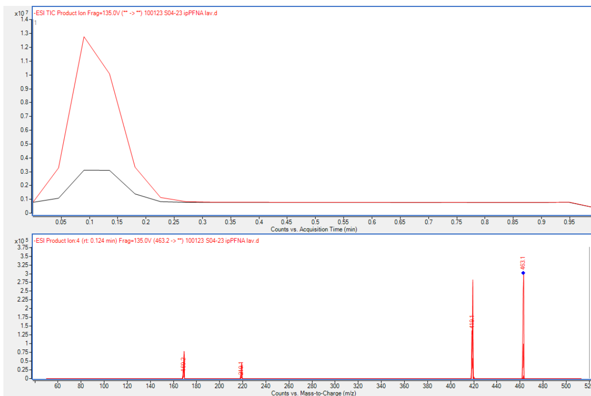
Figure D.2. MS optimization for ipPFNA. Product ion scan, where red chromatogram is low CE, and blank is high CE. The mass spectrum results from low CE and product ions are visible.
