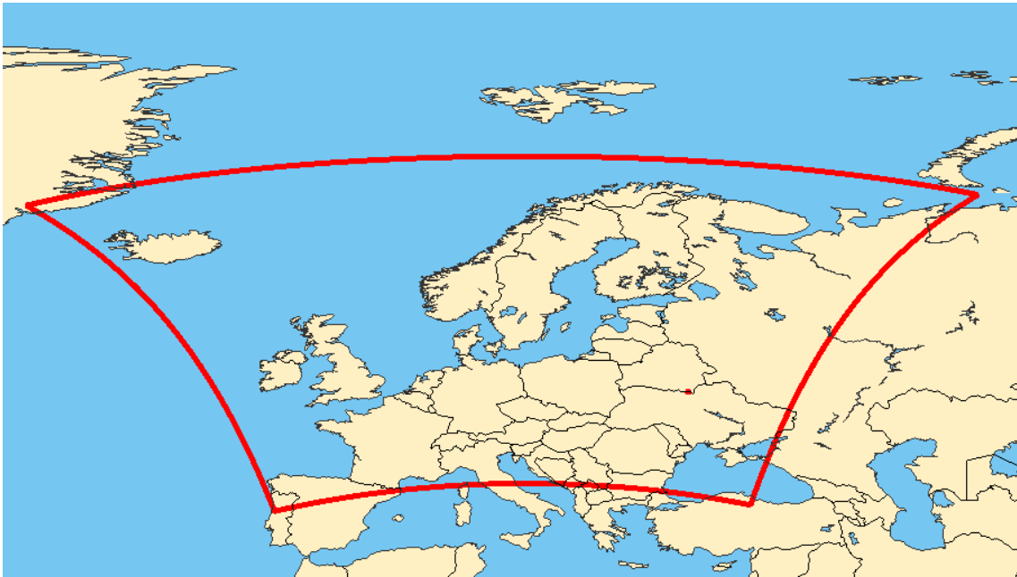
Figure 2.4: A Lambert conic projection shown on a geographic projection representing the model area for the hindcast looked at in this thesis. Retrieved from Diana
