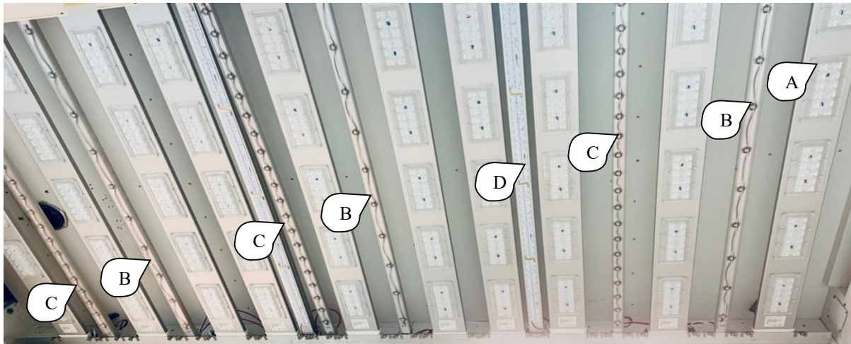
Figure 3.1. Light integrated in the CONVIRON growth chamber; white LEDs (A), red LED (B), and far-red LEDs (C and D) in the growth chamber.
