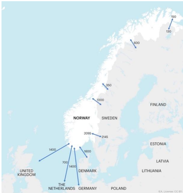
Figure 4: Map of Norway's electricity transmissions showing grid capacity of interconnectors in megawatts (IEA, 2022b).
