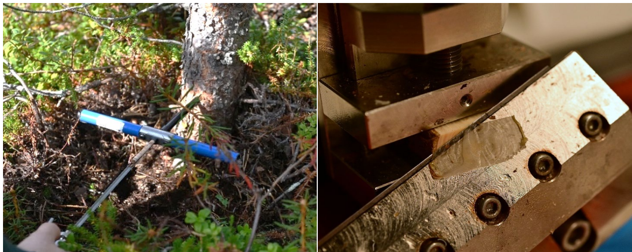
Figure 4 On the left, the coring near the base of a young tree with an increment borer. On the right the slicing of a sample using a microtome. Photos: Author
