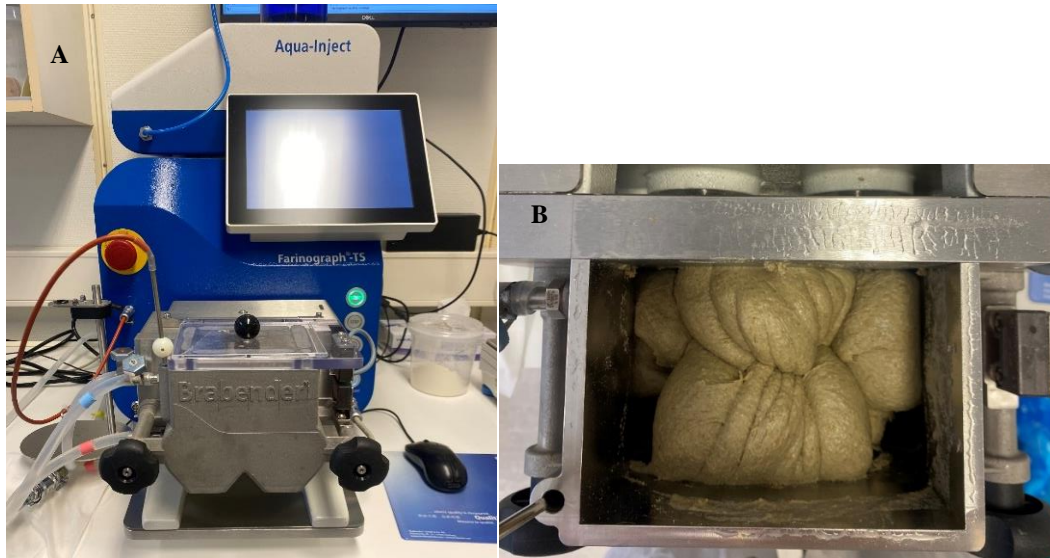
Figure 5. (A) Farinograph and (B) dough with fermented A. esculenta after 20 minutes of mixing.
