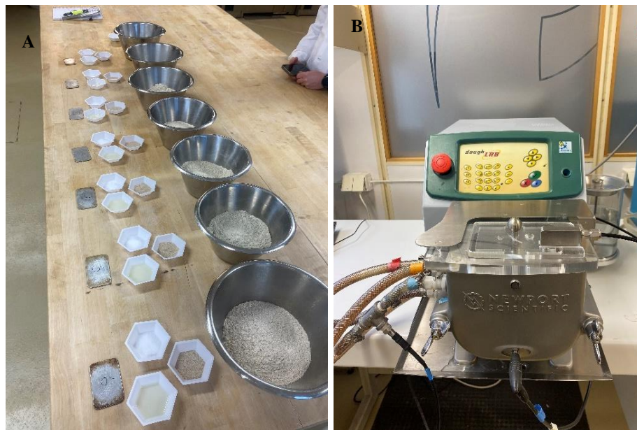
Figure 9. (A) Sample material used in dough and (B) DoughLab used for dough mixing.
