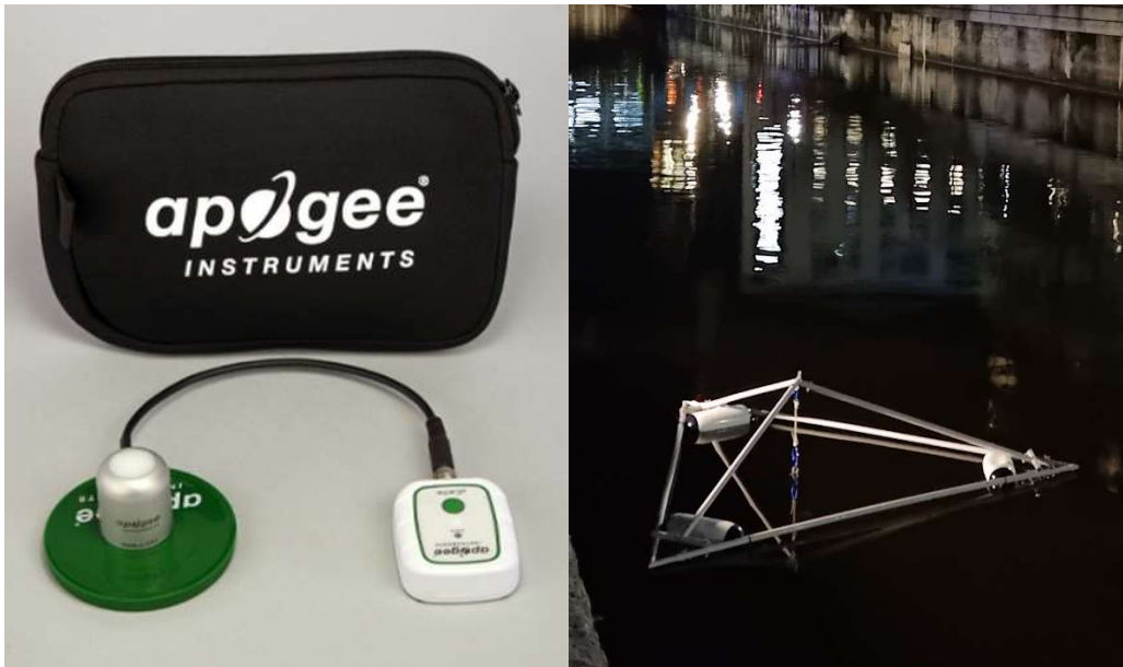
Figure 2. On the left the PAR-sensor (Apogee Instruments, USA) is shown, which was used to quantify underwater light. On the right the constructed float with the submersed PAR-sensor connected to the float with carabin hooks and thread is shown.
