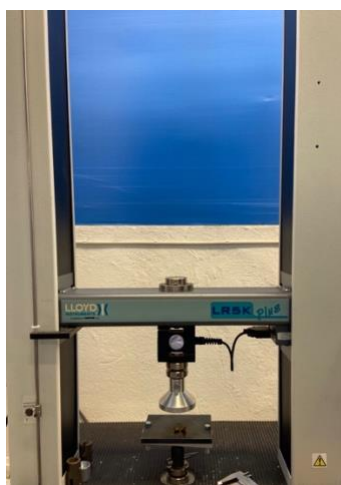
Figure 14 Lloyd hardness tester in Nmbu
