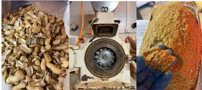
Figure 3 Peanut shells, Small Batch Grinder, Peanut Fiber
