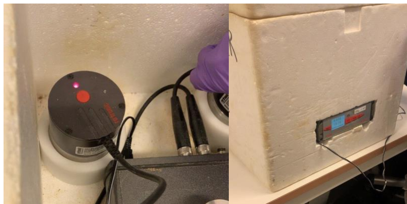
Figure 12 Inside layout of the A_w analyzer. Figure 13 A_w analyzer in Fôrtek
