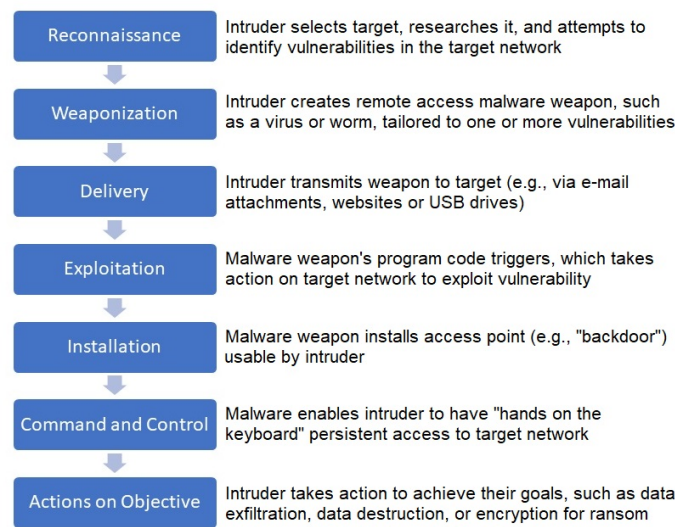
Figure 2. Cyber Kill Chain is a cybersecurity model that discovers the phases of a cyber attack, recognizes vulnerabilities, and supports security people to encounter the attacks at every step of the chain.
