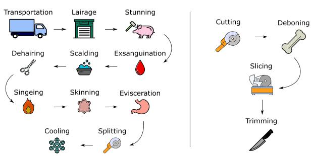
Fig. 2. A typical sequence for primary and secondary meat processing.
