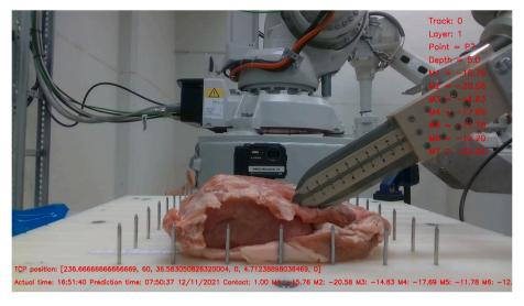
Fig. 11. Parameters read from the sensorised knife described in Mason et al. (2022) overlayed with image from camera.
