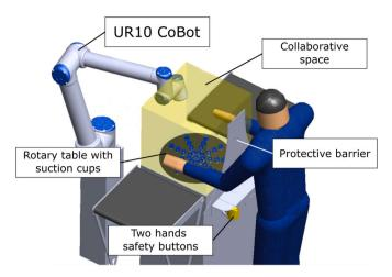
Fig. 9. An example of a cell based on HRC approach, for secondary meat processing in collaborative space (yellow cube).
