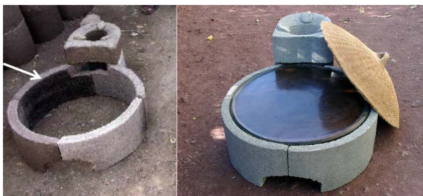
Figure 1. a) Mirt stove without Injera baking plate; b) Mirt stove with injera baking plate
