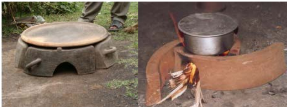
Figure 2. a) Gonziye stove set up for baking injera; b) Cooking with Gonziye
