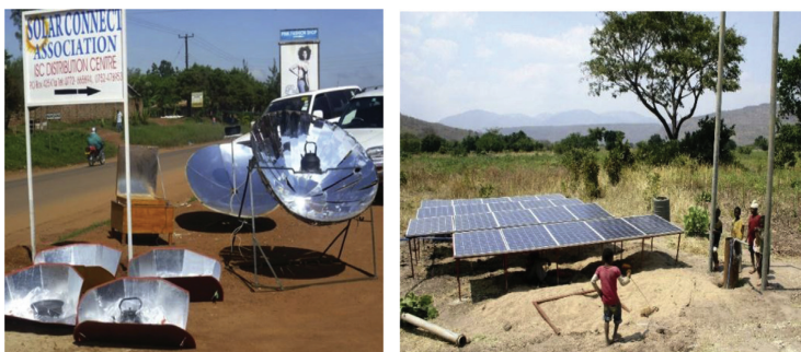
Figure 5. (Left) Solar cookers at Solar Connect distribution center in Kampala, Uganda (SCI [78]); (right) Solar PV water pumping in Tanzania (Solar Hope Foundation [79]).
