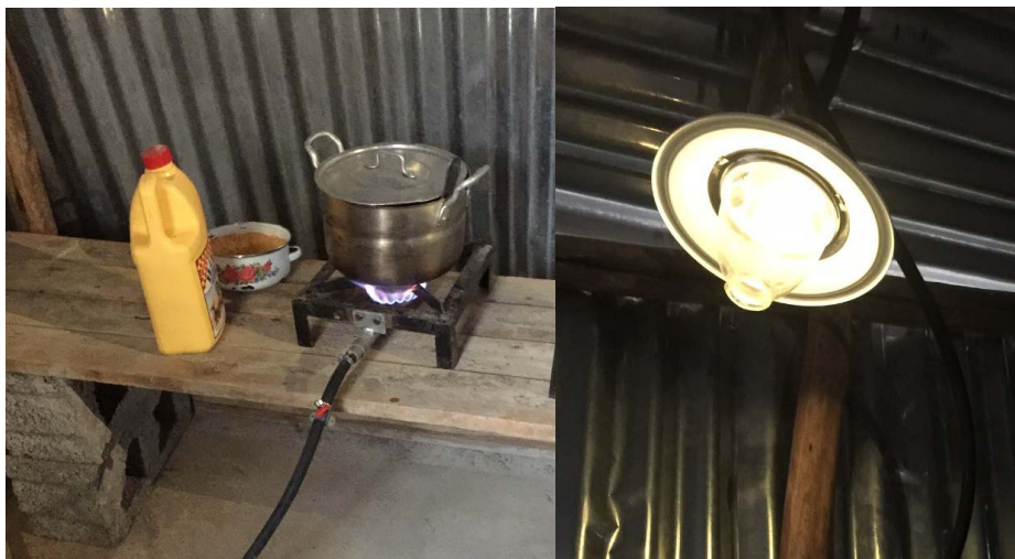
Figure 2. A typical biogas stove and lamp in rural Ethiopia (Photo credit: KG.hiwot)
