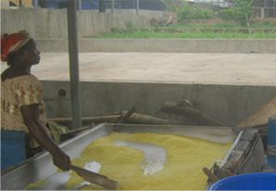
Figure 6.1: A garri processor frying provitamin A gari (Olaosebikan et al., 2017)
