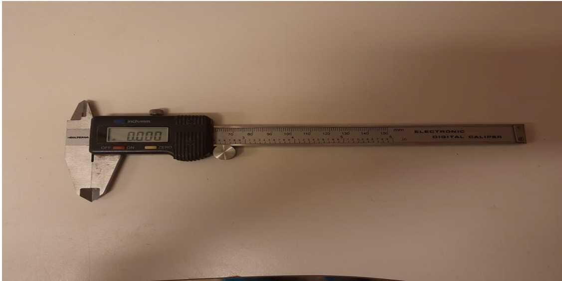
Figure 13. Vernier caliper used for length and diameter measurement
