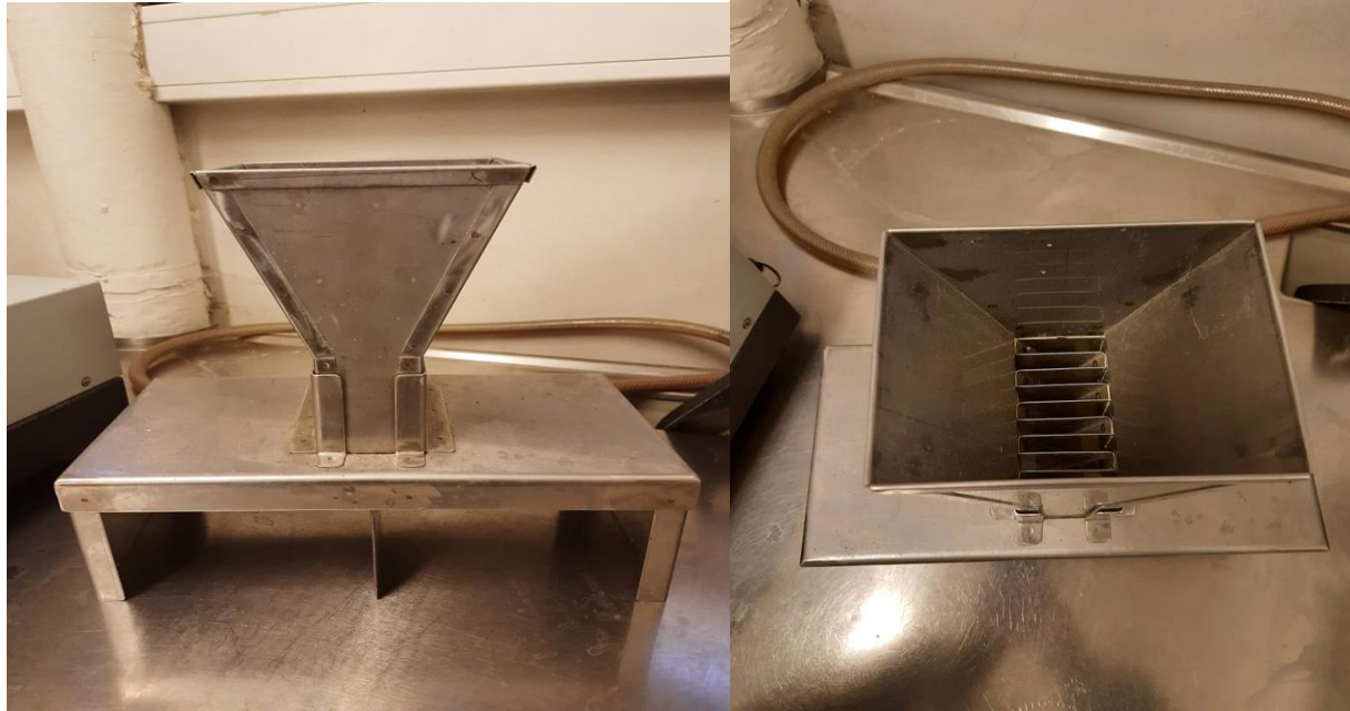
Figure 11. Sample divider for taking representative samples
