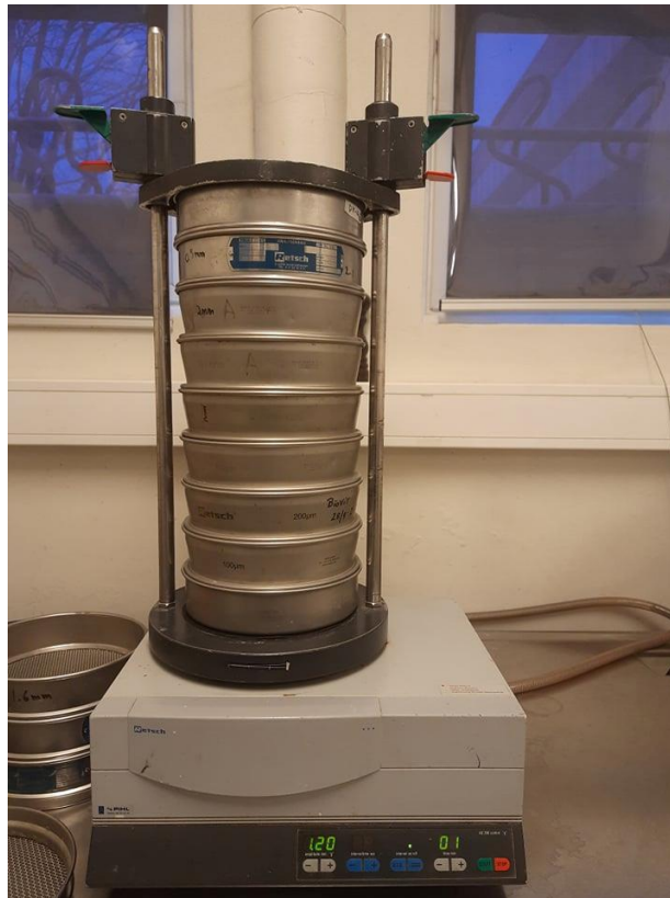
Figure 15. Retsch analytical sieve shaker with sieves and lid for dry sieving
