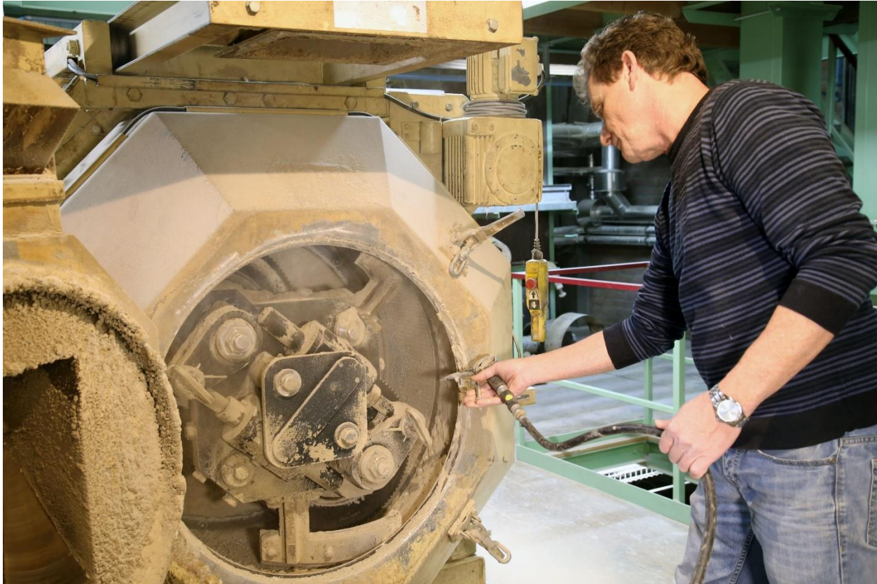
Figure 5. Pellet mill die chamber
