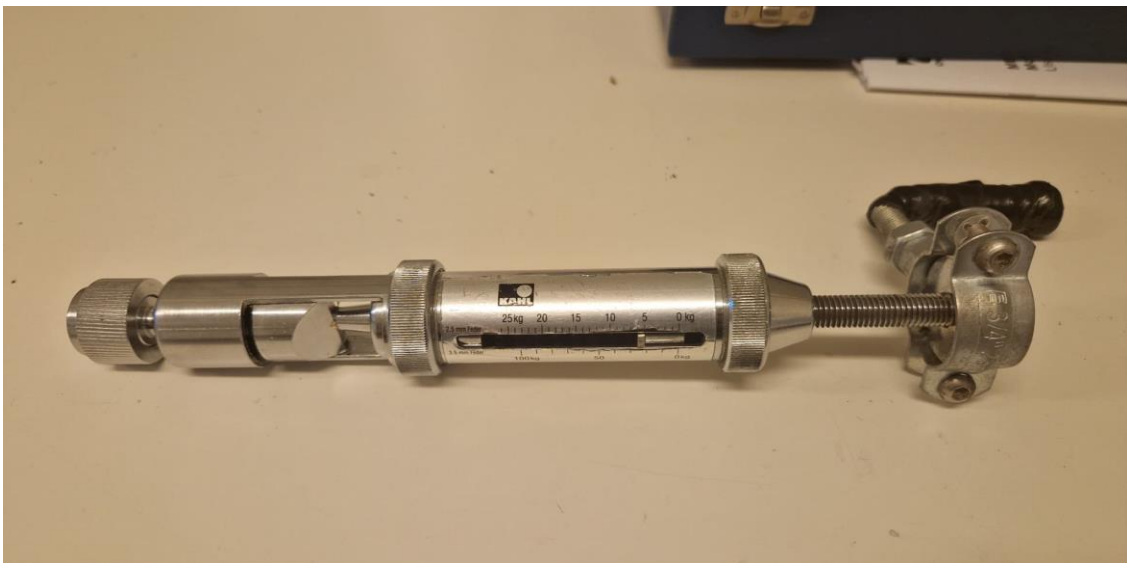
Figure 14. Kahl-hardness tester for pellets hardness measurement
