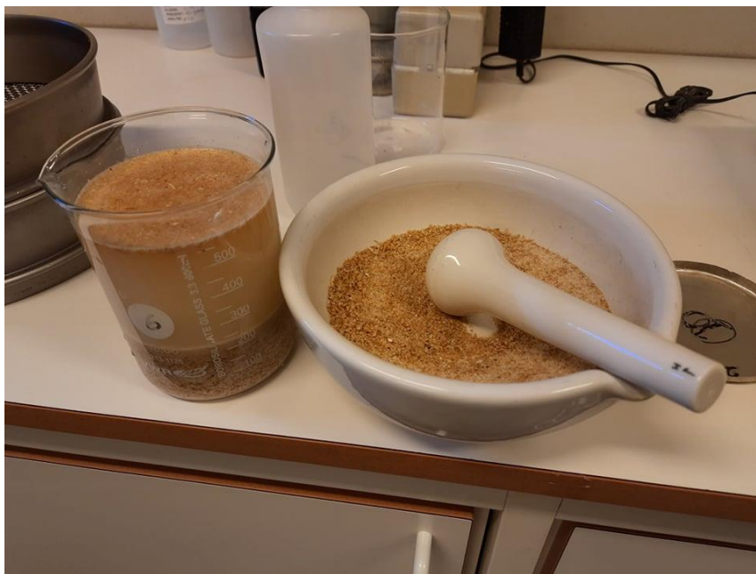
Figure 16. Beaker with dissolving pellets and mortar and pestle with ground sample for dry matter analysis
