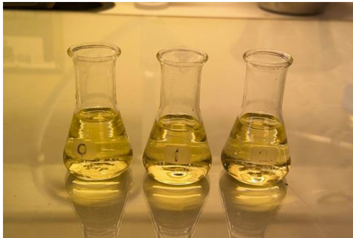
Figure B.8: Samples before reading in spectrophotometer: 0- blank sample, 2 and 3- after adding all chemicals.
