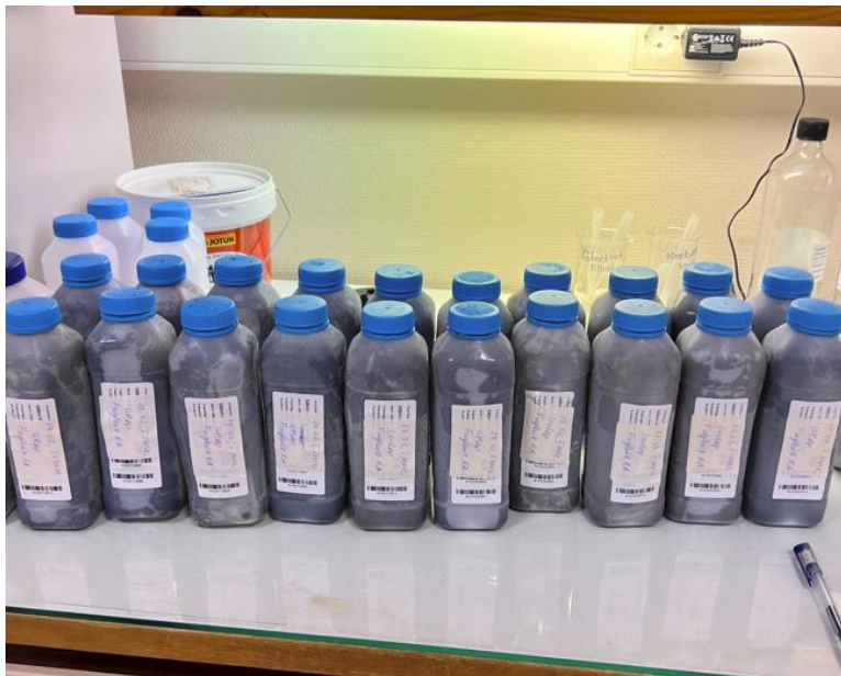
Figure 14: 8 plastic bottles (1 for raw sludge (influent) and 1 for digested sludge (effluent) from selected days were analyzed for PFAS.
