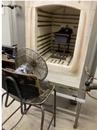
Figure B.16: Cooling station for the produced biochar.
