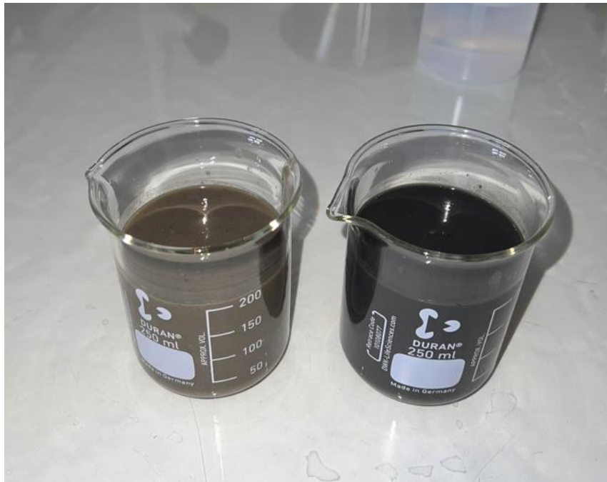
Figure B.2: The sample of raw sludge (to the left) and digested sludge (to the right).
