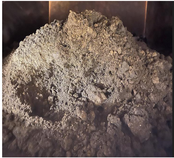
Figure 16: Dewatered sludge that is collected from the unloading containers.
