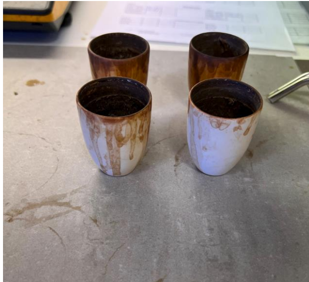
Figure B.3: Porcelain bowls: the first row is raw sludge and second row is digested sludge.
