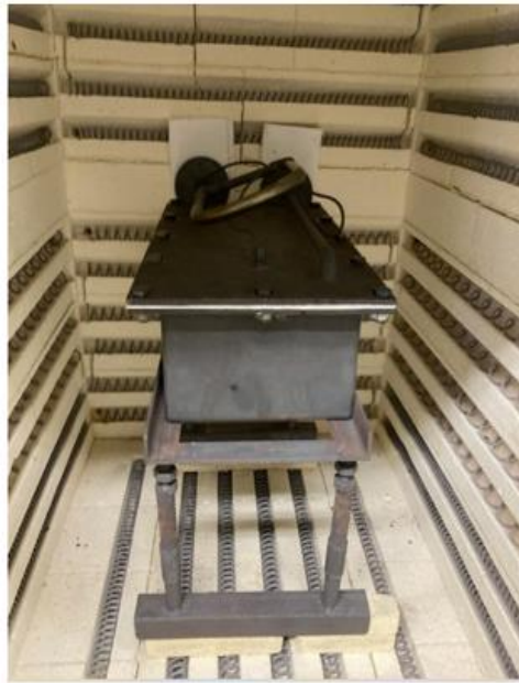
Figure B.15: Airtight furnace with nitrogen connected to it for performing of pyrolysis.
