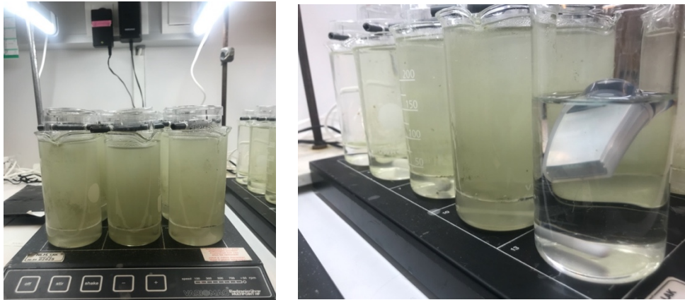
Figures 2 & 3: The photo on the left shows the test setup from the front. The picture on the right shows the other magnetic stirrer board with setup. The HOBO Pendant temperature and light logger is shown in the front on the board. Image: Thea Oma.
