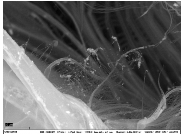
Figure 23: A SEM image of one D. magna exposed for tunnel particles from a 1200 mg/L starting concentration. Magnification: 1.39K X.
