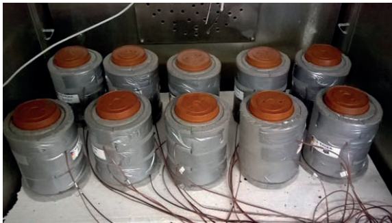
Fig. 1: Insulated soil columns in a Weiss freezing cabinet. The columns were placed on a polystyrene board. Thermistors were installed at two depths.
