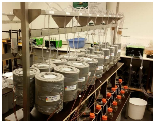
Fig. 5: Column set up in lysimeter lab during irrigations. Insulated, frozen columns in front, unfrozen columns in the back. Columns were connected to metal sieves and placed on funnels for collection of leachate.
