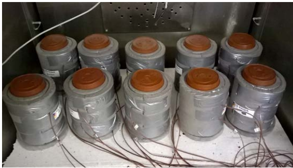
Fig. 3: Insulated soil columns in a Weiss freezing cabinet. The columns were placed on a polystyrene board and thermistors were installed at two depths.
