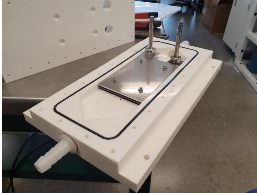
FIGURE 6 - INSIDE VIEW OF THE ECO EXPERIMENTAL UNIT, NEAREST NOZZLE IS THE INLET.
