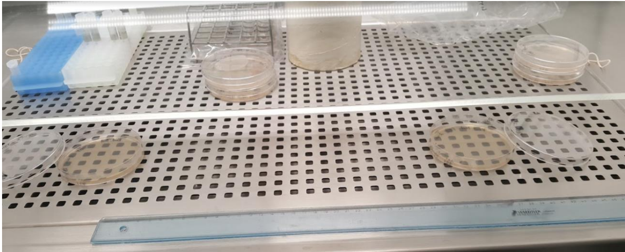
Figure 38: Setup of the contamination test. One plate was placed where secondary plates were processed. The other plate was placed 30-40 cm to the side.
