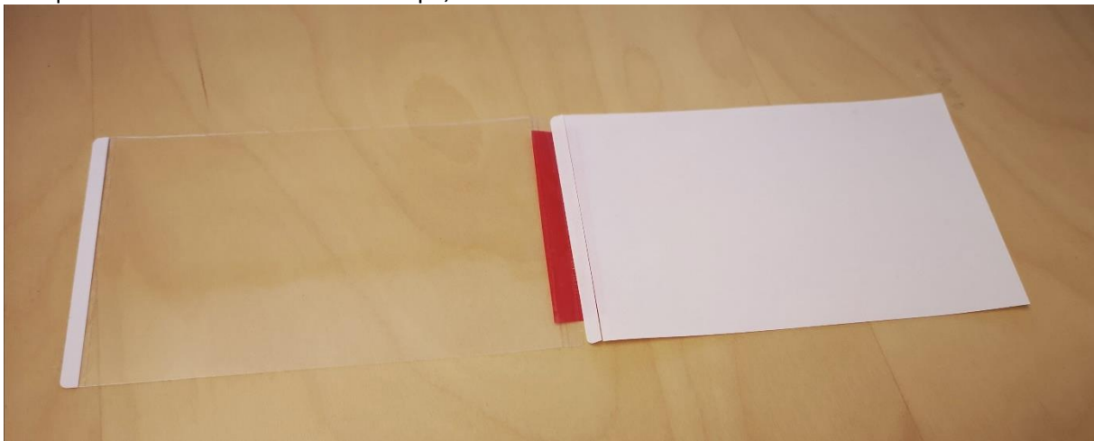
Figure1: The plastic film the way it is to be exposed. Keep the tape at the end on so it becomes easier to place the protective sheet back over the film after sampling.
